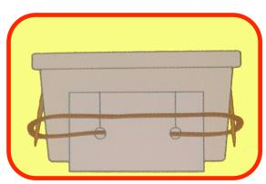
Slip the band through the slits into the holes. Then loop the band over the ends of the sticks.
