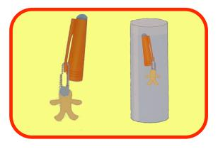
Cut a person out of the small plastic bottle and attach to the paperclip with blue tack. Test if the lid and person floats in a glass of water, if not remove some tack until it does.
