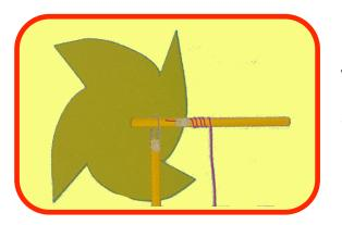
Tape the thread to the windmill straw. Wind the thread around it, leaving some hanging down.
