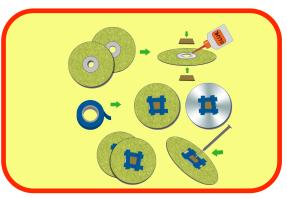
Put glue around the front and back of the holes of both CDs and stick the card squares over the holes on both sides. Secure it with tape. Pierce holes in the centres for the skewer.
