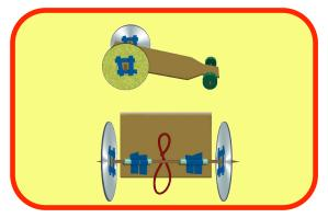
Loop a strong rubber band around the exposed part of the skewer. Tape it in place.
