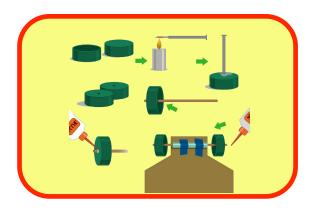
Heat the plastic lids to make them soft enough to push a nail through to make a hole for the skewer. Put the skewer through the front straw and attach the wheels and glue.
