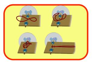
Pull the rubber band to the opposite direction so that it stretches sufficiently and then tape it in place.
